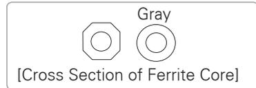
3 Use the ferrite core to reduce the electromagnetic interference in the PC audio cable. Wind the PC audio cable on the ferrite core thrice. Place the ferrite core close to the TV.
